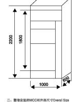
二、靠墙安装的MCC柜外形尺寸Overall Size of MCC Panel which install near the door
