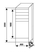
三、高墙安装的MCC柜外形尺寸Overall Size of MCC Panel which don't install near the wall
